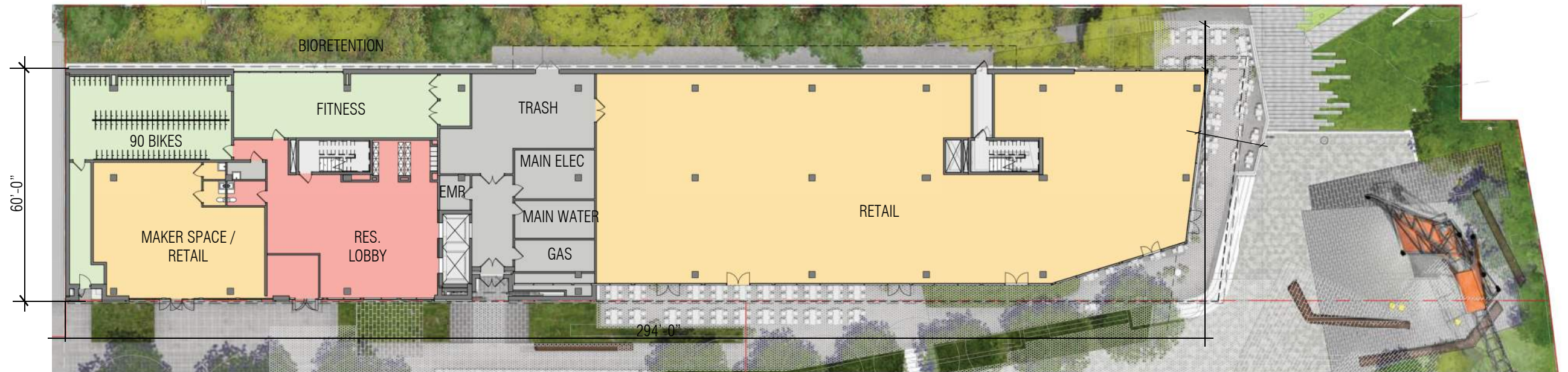
FLOOR PLANS - BUILDING B
